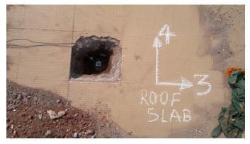
Accelerometer fixed to terrace slab
